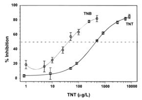
FIGURE 2. TNT and TNB standard curves for groundwater from Umatilla Army Depot. Standards were prepared in groundwater (85%) from Umatilla Army Depot. A minimum of three samples on different probes were tested for each concentration.
