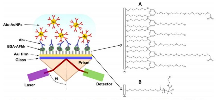
Fig. 1. The scheme of the optical setup and sensor chip with different surface architecture (A) mixed SAM and p(HEMA) brushes (B).
