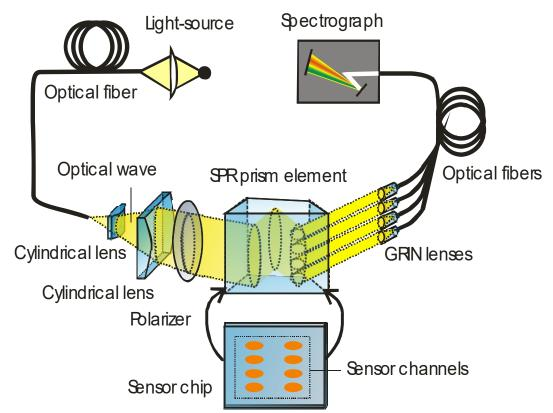
Example of wavelength division multiplexing of sensing channels combined with the using of multiple optical beams.
