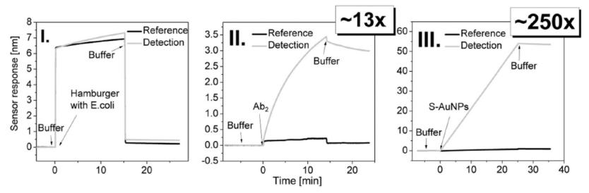
Fig. 2. Typical SPR sensorgrams obtained for the detection of *E. coli* O157:H7 ( $7.5 \times 10^5$  CFU/mL) in hamburger sample for each step of the detection assay as depicted in Scheme 2. The sensor response enhancement is given in the boxes.
