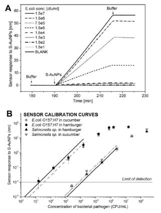
Fig. 3. (A) SPR sensor response to the binding of S-AuNPs in step (III) of the assay for the detection of *E.coli* 0157:H7 in cucumber sample. (B) Calibration curves for *E. coli* and *Salmonella sp.* in both hamburger and cucumber samples.
